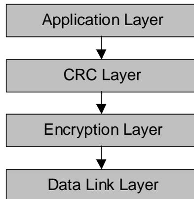
To send a message to e.g. a bill validator, we take the high level command consisting of a destination address, length field, command header and data bytes. A 16-bit CRC checksum is calculated and added into the structure. This is then encrypted and passed to the UART which adds in start and stop bits for transmission. The message is then sent to the peripheral device which performs the operation in reverse.
